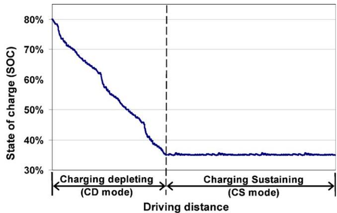
Fig. 1. Typical SOC of a range-extended PHEV.
